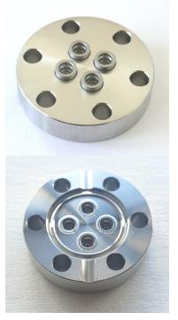
4 off SMP double sided feedthroughs on a DN16CF flange, shown from air side and vacuum side
